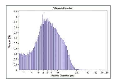
In multiple-aperture mode the software combines data from multiple series of analyzes using progressively smaller diameter apertures.
